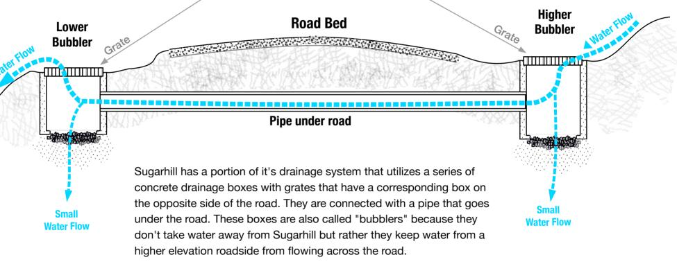
The higher ground bubbler takes water in that would otherwise cross the road then bubbles it up and out of the lower ground bubbler. The full intent of this is to keep water from flowing across and damaging our roads.
